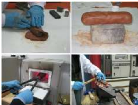
Figure 2: Clay sealing of a flat piece of Indian steel, annealing treatment for softening and later release from clay wrapping.
