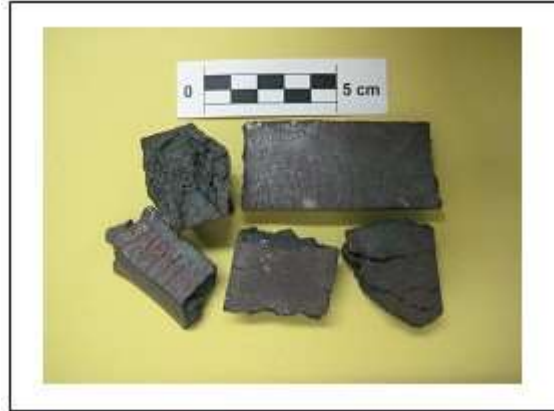
Figure 6: Macrograph of chunks of Damascus steel that broke during forging due to incorrect heat treatment.
