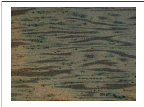
Figure 7: Detailed view of the ingot structure after sub-critical annealing followed by heat forging. Image obtained by means of conventional dark field microscopy. The image shows the structure of different sizes of carbides in alternate parallel sheets.
